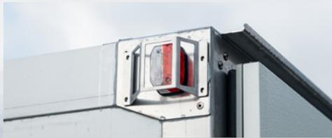
**Bumper protection made of stainless steel sheet.**
