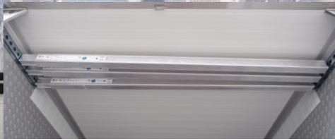
**Locking bar for load securing.**
