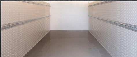
**Synthetic floor coating.** As a wear-resistant, slip-proof and absolutely leak-proof surface coating.
