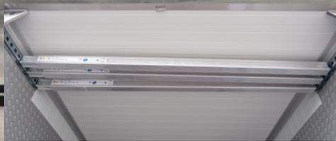
**Locking bar for load securing.**
